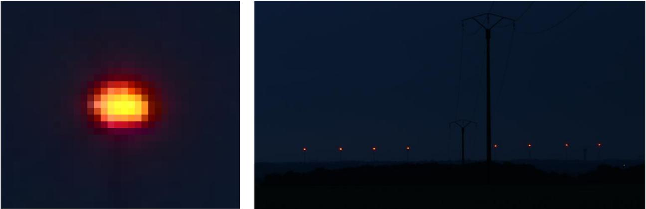
On the left is a detail of one of the lights. Knowing the distance, pixel dimensions and included angle the apparent size of the light is 18m across with a core size (near to maximum intensity) of 30% to 40% of the apparent size
