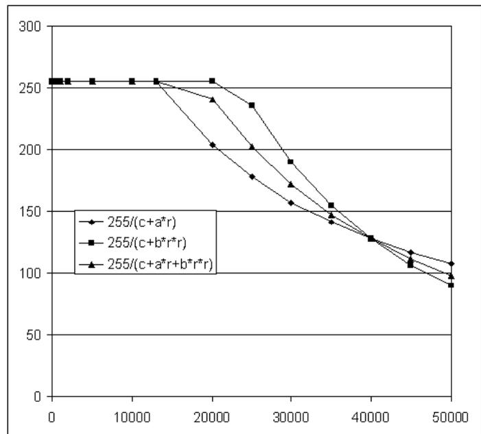
The spreadsheet AviationLights.xls gives this formulation for attenuation allowing you to consider the effect of different settings and choose the most appropriate for your photomontage. The intensity ratio is set as a percentage, the range is in metres and the constant should be between 0 and 1. In the Photomontage module you can also choose the amount of linear and quadratic attenuation to be used.
